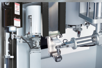
Intermediate guide and CNC electrode changer ATC (lh), CNC guide changer AGC (rh)
